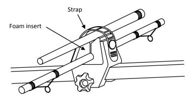
3. To carry oars/paddles/skis, remove the foam inserts and store in a safe place. Place oars/paddles/skis in the holder and tighten strap to secure as shown.
