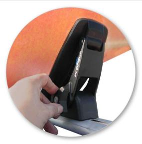
Cradles should fit hull closely to prevent movement during transport.
