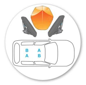
Cradle positions for narrow hulled kayak. NOTE: Kayak can be off centre on vehicle if required.
