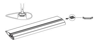
Tighten all screws to 5 Nm using the 4 mm Allen Key
