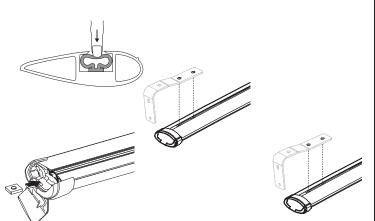
Noting the orientation of the Awning Brackets as pictured, check that Awning will not interfere with opening doors once fitted. If there is not enough clearance use the alternative orientation of the Awning Brackets. If there is enough clearance, secure the 2 x Awning Brackets to the M8 T-Nuts in the Crossbars by referring to Figure 1. Tighten to 4 Nm with 6 mm Allen Key provided or a suitable Torque Wrench.
