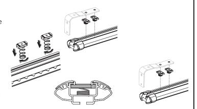
Noting the orientation of the Awning Brackets as pictured, check that Awning will not interfere with opening doors once fitted. If there is not enough clearance use the alternative orientation of the Awning Brackets. If there is enough clearance, secure the 2 x Awning Brackets to the M8 Spring Nuts in the Crossbars by referring to Figure 1. Tighten to 4 Nm with a 6 mm Allen Key or a suitable Torque Wrench.
