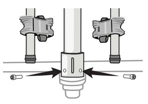
Secure mast to towball by tightening Capscrews with 10 mm Allen Key provided or a suitable Torque Wrench to 30 Nm.
