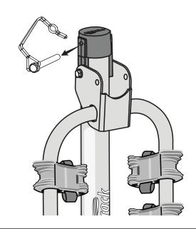
Remove the Locking Pin from the carrier.
