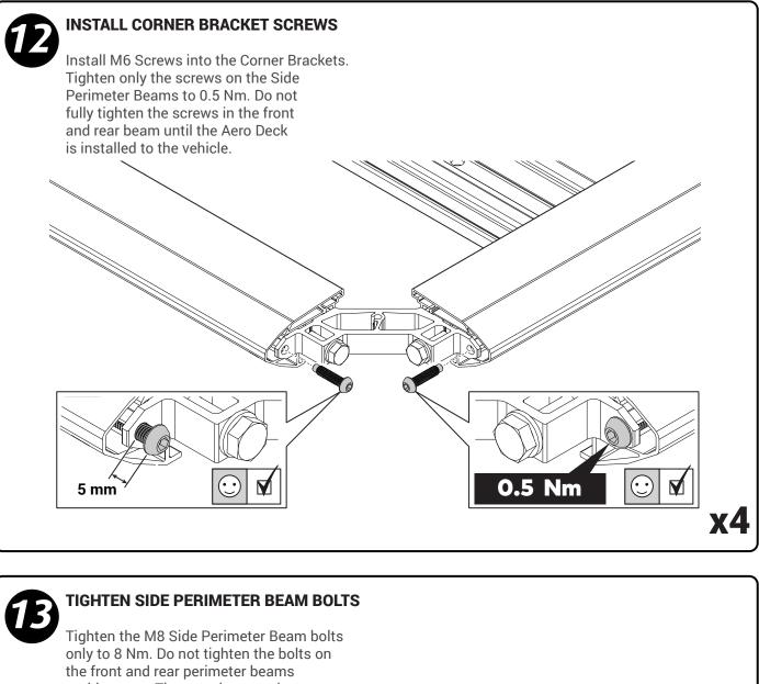
at this stage. They need to remain loose to be able to adjust the slats to position on the vehicle.
