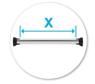
• Set bars to length so that the mounting holes will line up (refer to the crossbar instructions for crossbar adjustment).
