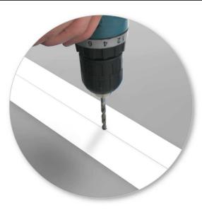
Use drill bit supplied, to drill holes in marked positions.
