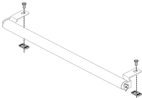
**3** Fit the split pins to the roller axle once the roller has been assembled to the brackets.
