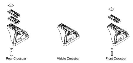
NOTE: Use the longer supplied capscrew for the rear bar assembly.
