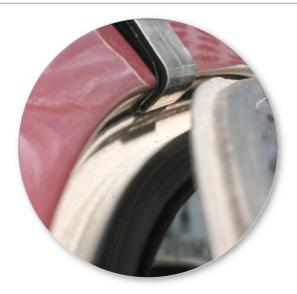
Ensure the clamps on the rear crossbar are fully engaged under the rear window aperture.
