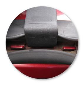
• Insert clamp into the mounting point.
