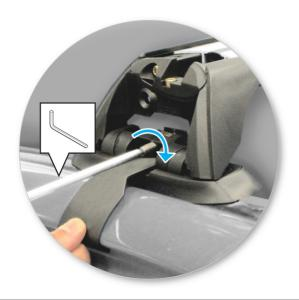
Progressively tighten the clamp block locking screws alternating from one side of the vehicle to the other to tension evenly.
