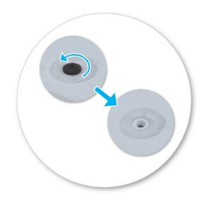
Remove fixed-point cover screws with 5mm Hex Key.
