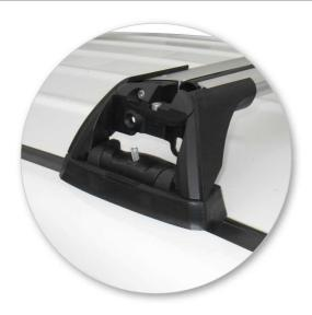
• Ensure that the bolt protrudes through the leg.
