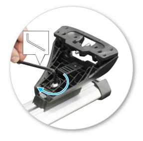
Using 5mm Hex Key supplied with this kit, fully tighten to 5Nm (3.7 ft lb) hand tight.
