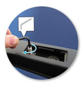
• Using 5mm hex key, screw M8 grubscrew into fixed-point, leaving 12mm (1/2") visible.
