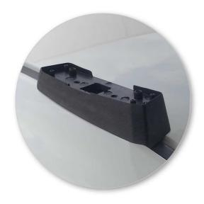
Place rubber pads (supplied with fitting kit) on the vehicle roof. Pad may vary in shape to that shown.
