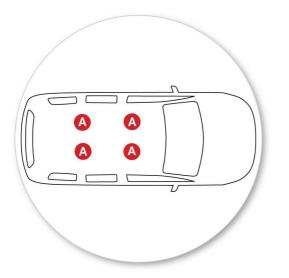
Use the following grubscrew lengths for each position: A = M8 x 80 mm (3 1/8")
